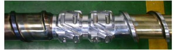
Standard Maddock screw : Local overheating is possible
