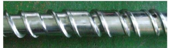
Upgraded screw : Suppress local overheating
